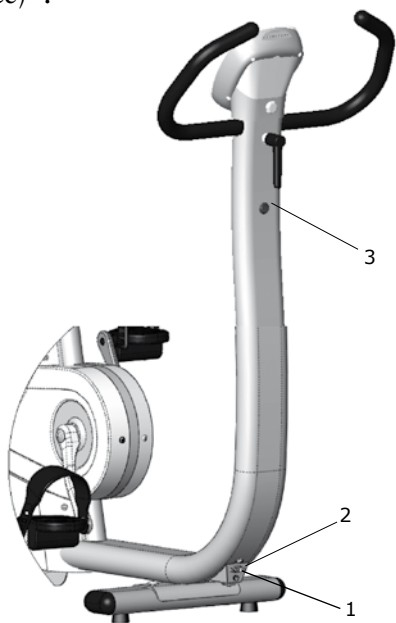
Fig: Connection 1) Power input 2) Serial port connection, external unit 3) Switch (on/off)
