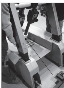
11. Open hardware bag "STEP 2". Commence, but do not tighten all the screws with washers on each upright using the smaller allen key (12 per side). You will tighten them later.
