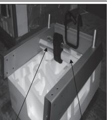
Tip: Keep the cross brace foam tubes on until you install upright to avoid accidental scratching. 4. Remove the rest of the components and place them on the box top or near by. Remove the base frame from the pallet and place it in the exact spot you plan to use it.
