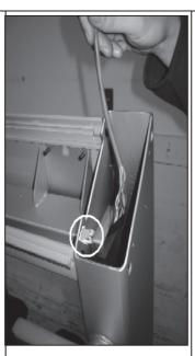
2. Clip the harness to the (2) harness clips along the frame. Once you have secured the harness to the clips, connect it to the female connector on the lower electronic board.
