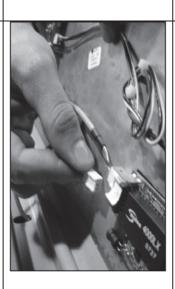
4. Connect the upper harness to the upper board. Center the membrane and pitch it back into place so that the velcro mates securely. Connect the main power cord to the front cover so you can turn the machine and verify all electrical connections.
