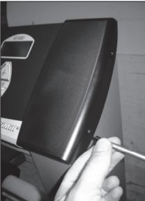
26. Open hardware bag "STEP 8" and use the allen key to fasten the rear step of the elliptical.
