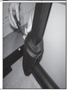
17. Slide the handrails into the upright fittings. Open hardware bag "STEP 5" and use the smaller allen key to commence the (2) screws on each rail. NOTE: There is a difference between right and left rails ("L" / "R" decals).
