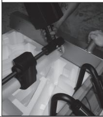
7. Open hardware bag "STEP 1". Use the big flat washer, lock washer and bolt to fasten the vertical stride adjustment members. After firmly tightening, cap the tubes with the large black dome finish plugs to conceal the hardware.
