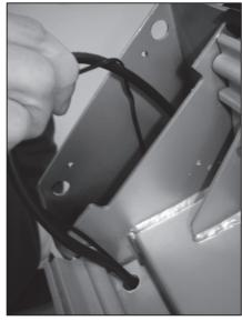
7. Grab the cable and power wires at the base of the upright through the access hole.
