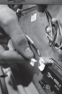
24. Connect the upper harness to the upper board. Center the membrane and pitch it back into place so that the velcro mates securely. Connect the main power cord to the front cover so you can turn the machine and verify all electrical connections.
