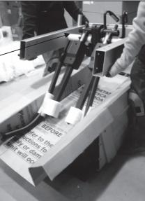
10. Carefully rotate the upright legs into the correct alignment and slip them into their respective black fittings on top of the frame. Once in, you can remove the protective cardboard and the plastic wrap / foam that secures the arms together (arrow pointing to it in picture).
