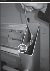
21. Clip the harness to the (2) harness clips along the frame. Once you have secured the harness to the clips, connect it to the female connector on the lower electronic board. TIP: If installing an LVS, install the Caddy (reading rack) now. Then LVS, then resume this assembly (step 22).
