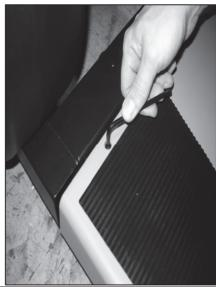
27. Check to make sure that the leveling feet below the step are firmly touching the ground to prevent any rocking.
