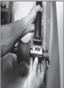
14. Open hardware bag "STEP 4". Connect the pedal arm to the vertical member. Slide the bolt in from the outside and tighten the nut very firmly. NOTE: There is a difference between right and left pedals ("L" / "R" decals).
