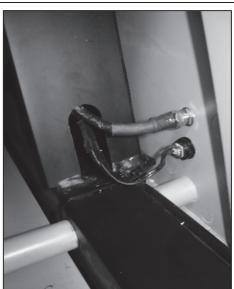
9. Push the cable and power wires (thin wire first) into the cable clip located underneath the control panel. This will prevent them from bouncing around during usage.
