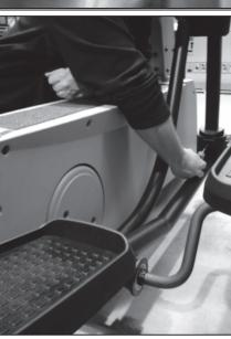
16. Use the remaining black screws in the hardware bag "STEP 4". Fasten the outside plastic joint covers.
