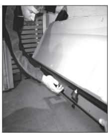
6. Slide the vertical stride adjustment members into the upright housing. DO NOT REMOVE the plastic wrap / foam that secures the two arms together. NOTE: There is a difference between right and left ("L" / "R" decals).
