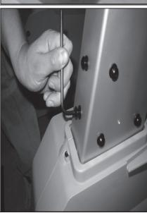
12. Using the rest of the screws in the the hardware bag "STEP 1", discard the protection caps and firmly fasten the moving hand rails using the bigger allen key. NOTE: There is a difference between right and left ("L" / "R" decals).
