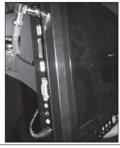
5. Feed the cable and power wires from the bottom of the tube into the left side of the control panel from the underneath.
