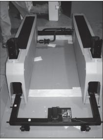
5. Check that all the leveling feet (6) are turned all the way up into the frame by tilting the machine and adjusting them as shown. Attempt to rock the unit back and forth to check for stability. If unstable, adjust the feet until it stabilizes.
