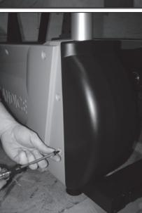
20. Feed the upright harness (found in membrane box) down the leg. Slide it all the way down until you can grab it at the base of the machine through the access hole. TIP: Once you grab the harness at the base, make sure to clip in the harness at the top of the upright to prevent it from falling down inadvertently.
