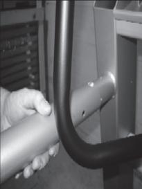
18. Use the remaining bolts in hardware bag "STEP 5" to fasten the bottom of the rail. Once you tighten these, finish tightening the smaller screws at the top of the rail. Once rails are tight, finish tightening the upright screws from assembly "Step 12" and the handrail screws from the previous step.
