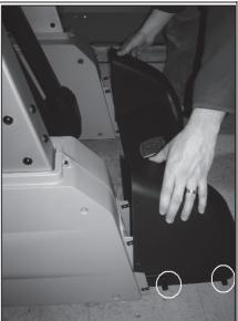
23. Place the membrane in the control panel and connect the two harnesses coming from the contact hand grips to the smaller board located on the far side of the membrane. The white connectors can go on either of the two available 3-pin connectors.
