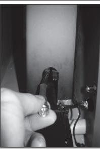
8. Connect the cable and power wires to their respective counter parts already mounted on the plastic covers right next to access hole.
