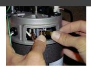
After the motor brush is seated back in and secured down, just pop the cover back on and repeat these instructions for the other side.
