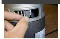
Insert the motor brush back Inside the brush holder.
