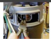
Connect the motor brush to the terminal using the needle pliers.
