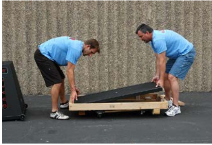
7. Carefully remove deck platform.
