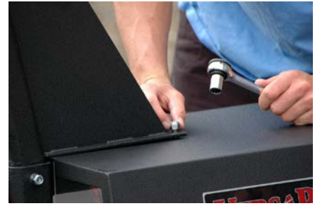
16. Use a 3/8-16 nut to secure the mast to the top of the housing cover.
